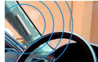
Should be fixed in an easy reception of cellular signal. It is important to ensure that the device is not fixed in metal parts of the vehicle and should be fixed preferably in the plastic. To avoid noise in the sound system, should be situated away from the radio and radio antenna.
