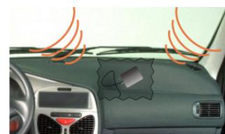
The antenna may be embedded in pieces of plastic, for example within the instrument panel. Should always be observed if there is no obstruction metal on it. You can also install in other locations on the vehicle, preferably near the glass.
